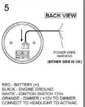
WHITE - IGNITION SWITCH 12V+ ORANGE - DIMMER / +12V TO DIMMER CONNECT TO HEADLIGHT TO ACTIVAE.
