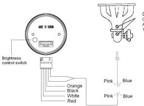
Drill a hole On either position And installing the 1/8 NPT thread Jointer
