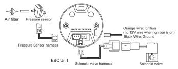
The harness and wires are designed to use with EBC only. Please do not use with other products or the product will be damaged.
