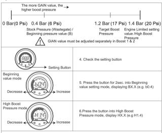
Enter into setting mode, press the ahead right button to decrease 0.1 bar, press left one to increase 0.1 bar No reaction within 5 or press the setting button behind the main unit to finish setting than
