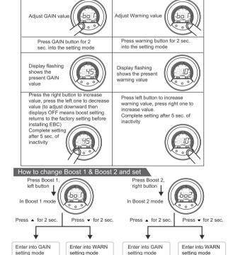
Once set, just need to press the left or right button to enter into the preset boost pressure of Boost 1 and Boost 2 mode
